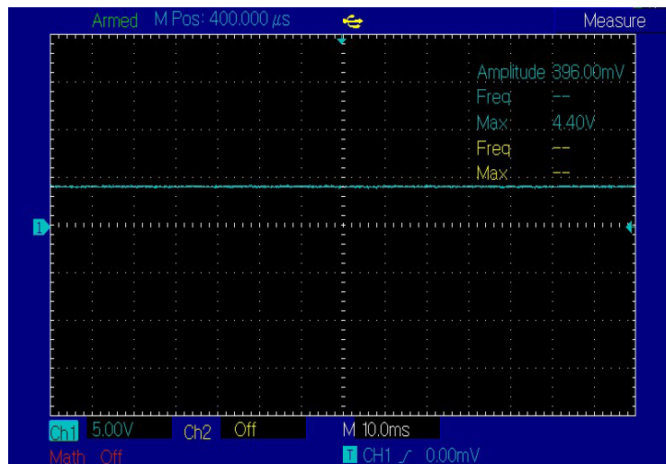
Fig. 15 Charging Voltage Waveform Under Solar Panel System
