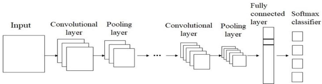
Fig 1. Structure of a CNN [15]
