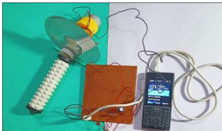
Fig. 4 Hardware Implementation of Medical Mechanical Mobile Charger
