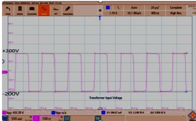
Fig. 5 Transformer Primary side voltage
