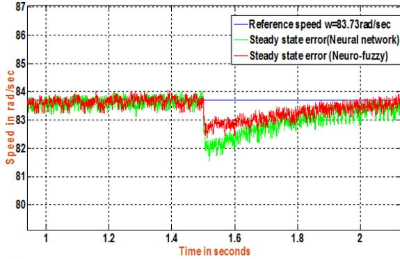
Fig. 13 Steady state error of the actual speed when reference speed  $\omega=83.73\text{rad/sec}$
